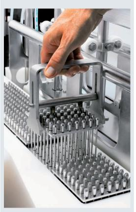
**Needle removal tool**Easy and quick needle removal.
